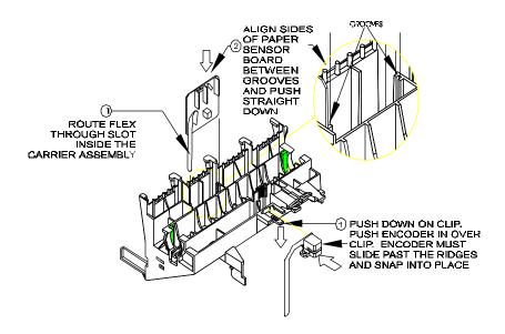
Figure 5-9. Paper and Encoder Sensor Installation.
